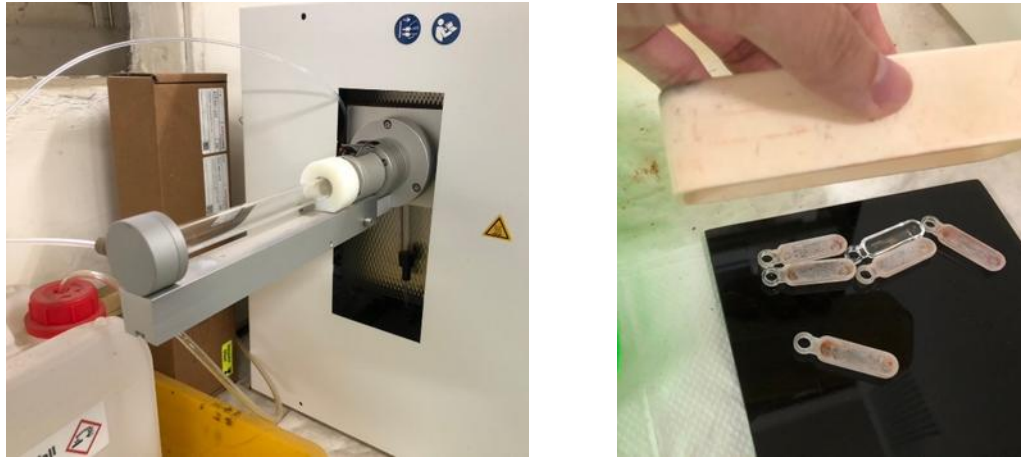
Figure. 8 Dry Combustion Method Operating Procedure (Source: Produced by This Project)
